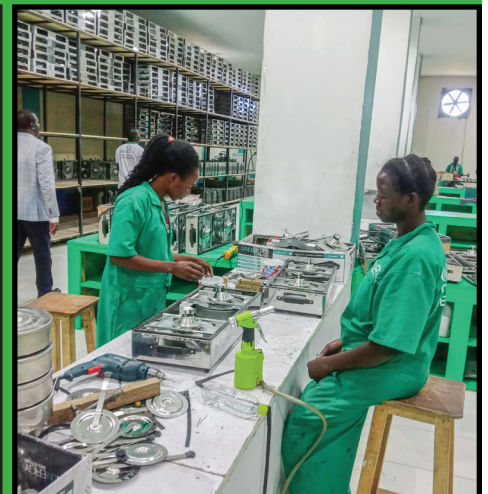
Employees of the factory at work, assembling the bio-stoves that use ethanol for cooking. Photo by ARU Reporter.
